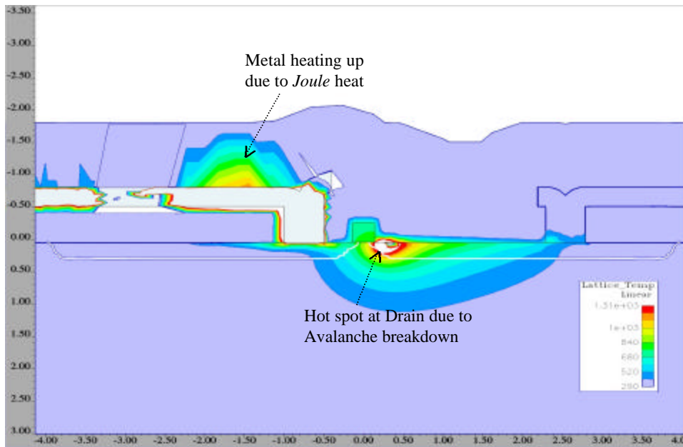
Fig. 19b Enlarged image shows thermal defect in the metal layer as well as in the Si channel.
